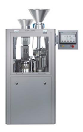
The NJP-200C automatic powder capsule filling machine, as a perfect upgrading alternative for semi-automatic capsule filling machine, has been widely used in Pharmaceutical, medicine, and chemicals (powder, Pellet, granule, pill), also can be used to fill vitamin, foodstuff and animal drug, etc.
