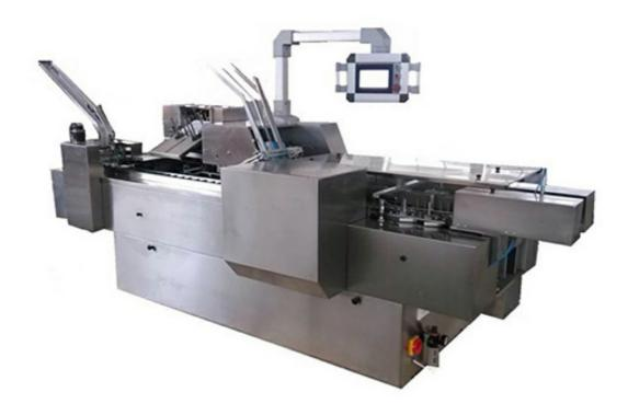
Used for cartoning packing process for blister, bottle, tube and etc.
