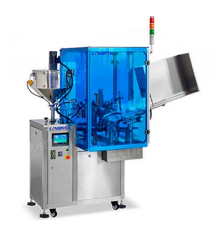
The automatic aluminum tube filling machine is suitable for paste materials, ointment, adhesive, AB glue, epoxy glue, skin cream, hair dye, shoe polish, toothpaste and other liquid. The outrigger mechanism of the machine is made of aluminum alloy and stainless steel, equipped with dust cover.
