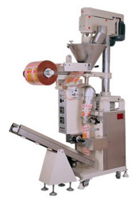
Vertical Machine SP-203BSA suited for filling food, pharmaceutical chemicals, and agricultural chemicals. 35 - 65 angle of repose or particle allowed break, and other non-free flowing powders.
