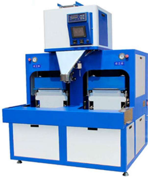
This machine consists of one set linear weigher for weighing and filling, one set vacuum packaging machine, one set take-off conveyor, manual put the bag on weighing machine discharge mouth, the weigher automatically weighing and filling, then manual put the bag on vacuum device for automatically vacuum and sealing. It is suitable for granules, such as: rice, miscellaneous grains, beans, cashew nuts, etc.
