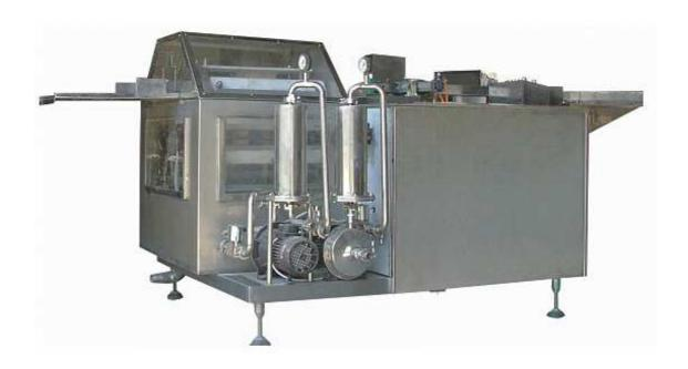
This machine is applied in clinical bottle and dropping bottle cleaning use to turn the drum frame, and provide a dish to provide the bottle, and be sent by stir the round bottle, turn the drum intermittent into the bottle, use again back to use the water (Or running water), go to leave the son water (or distilled water) and decontamination compressed air to hand over for flush to complete the bottle-water.
