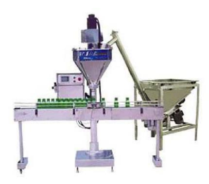
This powder filling line (automatic powder filling machine) is mainly used to fill a wide variety of powder materials that are easy or difficult to flow, such as veterinary drugs, powder additives, sugar, soft white sugar, glucose, monosodium glutamate, solid beverages, pharmaceutical solids, toner, powder, pesticides, dyes, flavors, fragrances, and so on.
