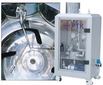
The WIP, (Washing In Place) system automatically cleans each part of the coater. 5 nozzles are equipped for the cleaning of the in/outside of the coating pan and the in/outlet air duct lines. The mains water, detergent or purified water can be selectively sprayed for cleaning according to the contaminant condition after production.
