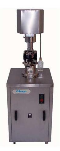
The semi automatic cap sealing machine is precision built on sturdy welded steel frame completely enclose in stainless steel sheet and doors are provided to facilitate the servicing of machine. Machine is motorized incorporating rotating threading & sealing rollers, for threading & sealing of ROPP cap.
