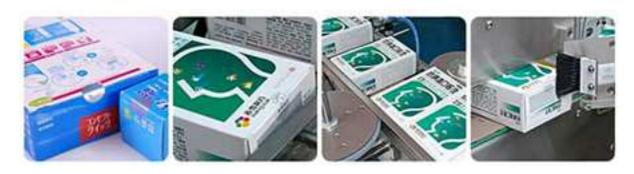
A928 is designed for seal labeling on two opposite corners of small pharmaceutical cartons. The system provides complete process in carton separation, hold-down stabilizing, labeling, corner wrap adapting, and missing label detection and rejection to ensure perfect output quality. It is an ideal equipment to connect to high speed cartoners for subsequent corner sealing of the cartons at the end of the line.
