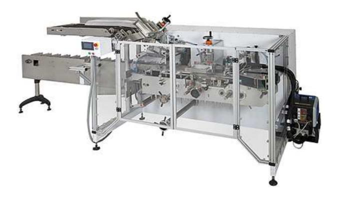
The new series carton machine built with "BALCONY" design, allowing the mechanical working parts separated from the packaging area. It respects the present accident prevention maintenance and hygienic laws.
