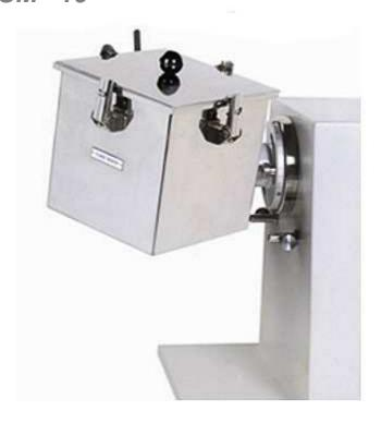
The Mixing movement of the product in the mixer is deflected and interfered by three mixing rods made of stainless steel. The cube Mixer is a based on a movement, which through its tumbling effect produces in the shortest possible time a homogeneous mixture. The product to be mixed is treated very gently. The cube Mixer can be attached to the universal gearing. The housing is manufactured from stainless steel. This Attachment is Suitable to Attached in our Both Main Drive.
