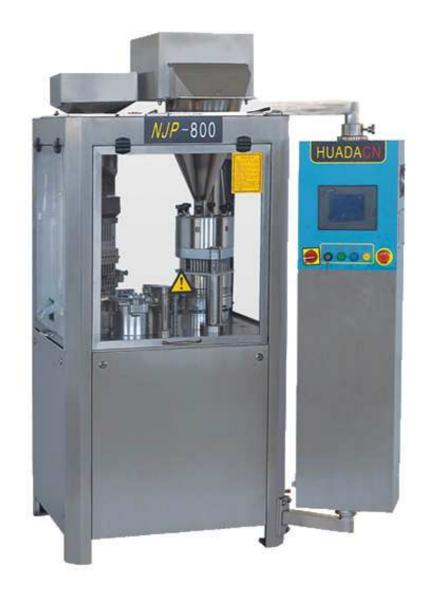
This machine is fully automatic capsule filling machines. It is suitable for capsule size from 00#, 0#, 1#, 2#, 3#, 4#.
