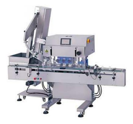
SXGJ130 high speed rubbing machine is adapted to cap various kinds of bottles (round, oblate and square bottles). It is widely used in medical, healthy, food chemical and pesticide industries.
