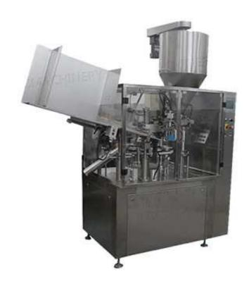
A soft tube filling and sealing machine is mainly used for plastic tube filling and sealing. It has been widely used in the fields of pharmacy, cosmetic, food and chemical etc.
