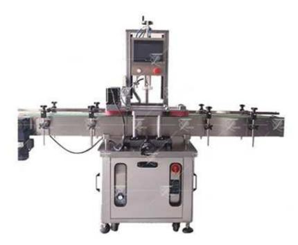
This machine is a fully automatic cap screwing machine. It is widely used for bottles with pump, duck-billed cap or round cap, etc
