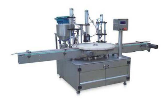
Filling and capping machine is one kind of automatic production equipment, it's suitable for different viscosity liquid. Pneumatic piston type filling, volume measurement. High precision and efficient.
