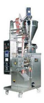
The machine is suitable for packing non sticky, bulk or granular material, such as medical pills, food Stuffs, plant seeds, washing powder, coffee, sugar, desiccant etc The integrated processes of bag making, measuring filling, sealing cutting, counting and hot pressing codes can be done automatically. Packing material include several kinds of heat seal lamination, such as PET/plated AL/PE, PET/PE, PAPER/PE, NYLON etc.
