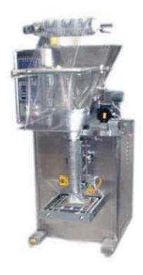
This machine is widely applied for food, pharmaceutical, and chemical products in mesh size range from 120 to 400, such as milk powder, soya powder, cosmetic powder, slimming tea, medical powder, etc.
