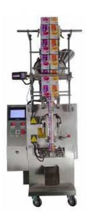
This machine is applicable for powder packaging Be used for packing powder in field of food, medicine and chemical
