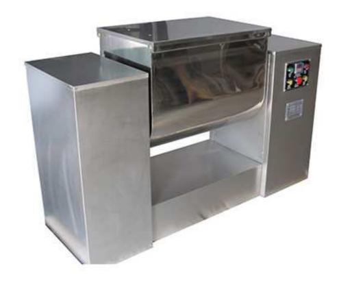
Trough Type Mixer is suitable for Pharmaceutical, Chemical, Food and other industries, primarily dealing with evenly mixed powder or pasty materials. The machine works by adoption of mechanical drive as it can improve the quality of each batch of mixture with high degree of uniformity.
