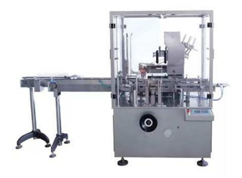
HTZH-80 automatic cartoning machine can be applied to bottles, column product boxing. The products will arrange into tray automatically by the bottle arrange machine. The tray will be separated one by one, and then conveyed to the loading station of the arrange machine, then, bottles will be packed into tray automatically. Then, conveyed to packing machine to complete the tray into box functions.
