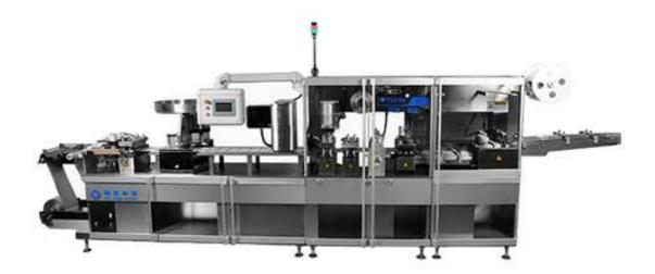
Fission Combination Structure: accessible to elevators or renovated clean workshops. Length of stroke by digital control, running speed directly set on human-machine interface according to the material feeding conditions. Printing Register, Missing Pills Rejection Device.
