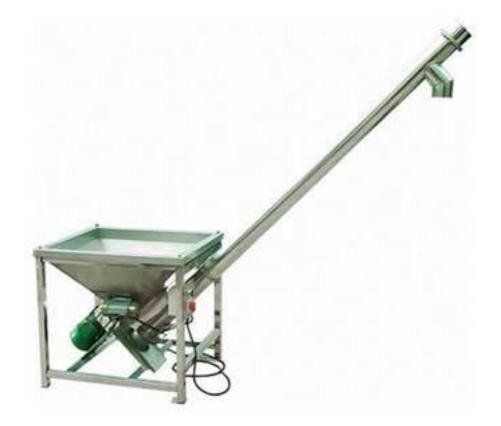
Vibrating powder feeding machine (also named Screw Conveyor Feeder) is suitable for feeding powders mixed powders into the hopper of auger filler.
