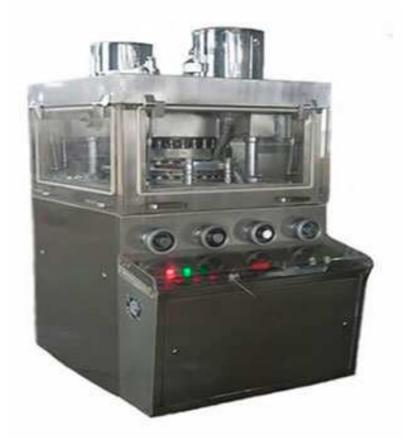
This machine is a kind of double press automatic rotary, press continuous machine, press granulate material to tablet.
