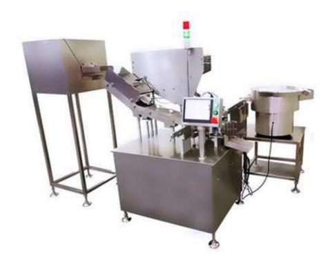
The BSP-40A Tube Filling Machine for Tablet is applicable to the packing bigger and thinner tablets which are orderly fed into bobbin bottles in single row in an overlapping way. The device utterly adopts a PLC for centralized control, it is verified in fiber and photoelectric detections and other kind of detections to have steady performance and reliably automatic operation. It can automatically give alarms and shut down in case of no tablets, bottles or covers.
