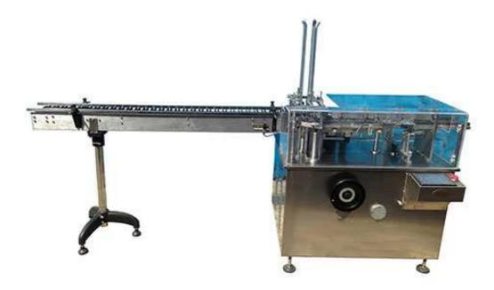
The equipment is mainly used ointment class (aluminum bottles and plastic bottles), automatic cartoning, The machine automatically complete manual folding carton forming automatically open a ointment vial automatic cartoning, the three unified completed action function, batch number can be automatically printed on the box side.
