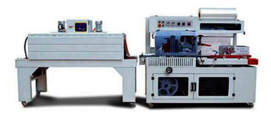
PZS-650L automatic heat shrink packaging machine is a fully automatic unmanned operation "L" automatic shrink packaging machine, widely used in food, pharmaceutical, daily chemical, hardware, electrical and other industries, especially mass production. Packing flow operation, high work efficiency, automatic film feeding and punching device and manual adjustment of the film guiding system and manual adjustment of the feeding platform for different widths and heights.
