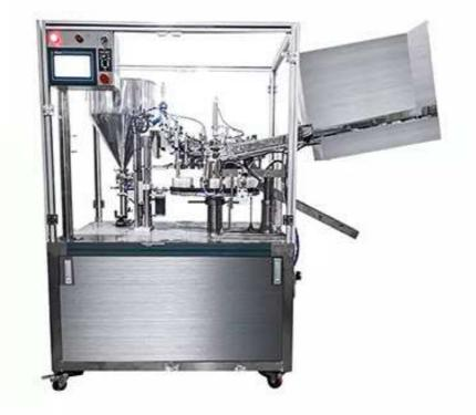
Mainly used for packaging materials with aluminum tubes. This machine is widely used in packaging in the pharmaceutical, daily chemical, food, chemical and other industries. Such as ointment, toothpaste, epoxy glue, 502 glue, hair dye, and other liquid or paste-like materials filling and sealing.
