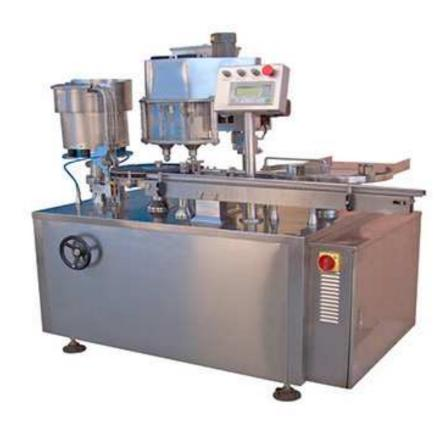
Vial injection filling production line project (GMP) is a kind of screw type sterile vial powder filling machine our company has newly developed. It adopts two track, cylinder positioning, 2 head screw filling and 2 roller stoppering. The servo motor controls the filling auger precisely.
