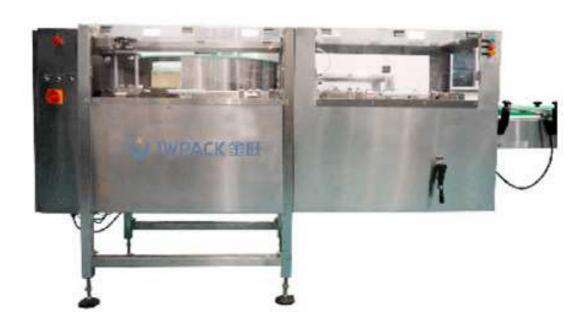
LP-100B Automatic Bottle Unscrambler is making up with the bottle elevator, unscrambling rotary plate, bottle rejecting devices, unscrambling and electrical control cabinet. It can arrange the disordered empty plastic bottles into good order. The machine is with the features of compact structure, simple operation, mature technology and stable running and operation.
