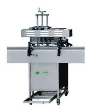
Utilizing electromagnetic principle, high frequency signal after amplifying output through interaction coil, as the container with compound aluminum tinsel in inner cap pass through the interaction coil, immediately generate eddy current heat, make the aluminum tinsel side glue closely with bottle mouth, reach the purpose of airtight sealing.
