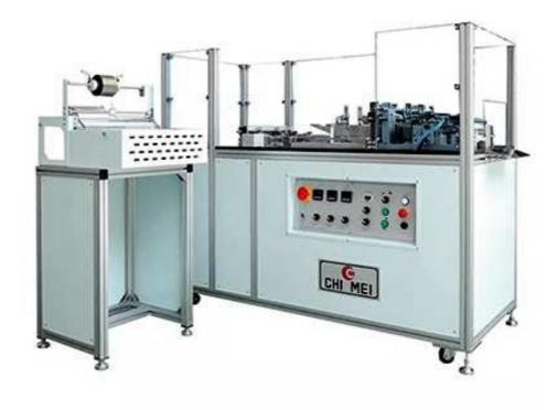
This model is combined with "manual cellophaning machine (PM-205A)" and "automatic angle banding machine (PM-207A)", which is suitable for sample proof packaging and is also suitable for normal packaging production.
