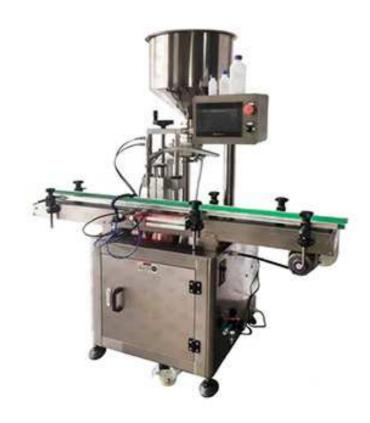
Our automatic single head liquid filling machine is made of 304 stainless steel or 316L stainless steel. It has easy structure, great injection precision and convenient operation. It is widely used in food processing with long service life.
