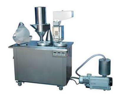
NJP-S semi-automatic capsule filling machine is suitable for filling various domestic or imported capsules. This machine adopts electrical, pneumatic joint control, and is equipped with an electronic automatic counting device, which can automatically complete the actions of capsule positioning, separation, filling, and locking, Reduce labor intensity, improve production efficiency, and meet pharmaceutical hygiene requirements.
