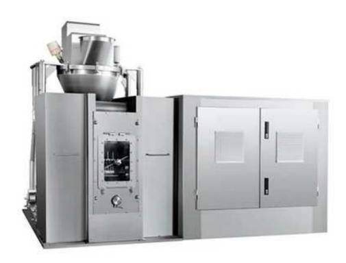
Dry granulation is widely used in pharmaceutical, food, chemical and other industries. It is especially suitable for granulation of drugs that are easily decomposed by moisture, easy to absorb moisture, sensitive to heat, and the particles can be used for densification to improve fluidity, tablet compression, Filling capsules and granules for bagging. This machine is especially suitable for mass production.
