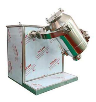
The working principles when the Pharmaceutical Manufacturing High Efficiency Mixer is in operation. Because of the running actions of the mixing tank in multi direction, the now and derision of the various kinds of materials are sped up in the process of mixing.
