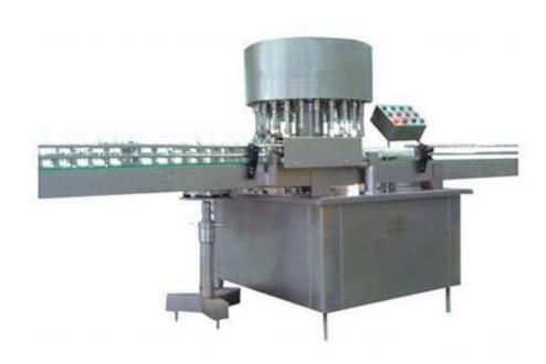
Mainly used for automatic stopper (including T type rubber stopper) and pressure stopper of infusion glass bottles.
