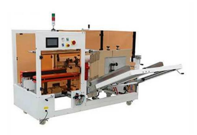
Carton erector machine ZF-K20TX, automatically opens the carton board, folds it into shape, and seals the bottom tape. The speed can reach 10 cases/min. Man-machine interface control, fault display, more convenient maintenance; automatic alarm for lack of material; feeding does not need to stop, does not affect production, and better improves production efficiency.
