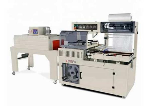
FL-450A semi-auto L-type sealer and BS-4522N shrink tunnel are suitable for packing boxes, toys, electronic bricks and so on. The two machines can pack the products with a layer of plastic film, which makes the packaging more beautiful and firm.
