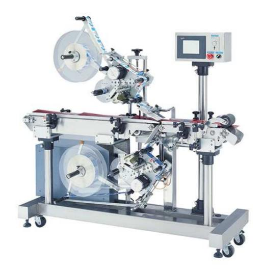
This machine is designed for top and bottom labeling on flat products. It can be incorporated with a line or operated individually.
