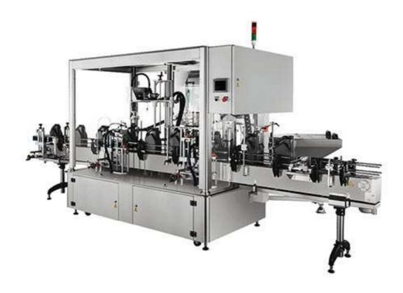
KWT-150 / 180 serials are cap chuck capping machine, the pick & place device which picks up the cap from the chute and places it on the container, then capping chuck tightens.
