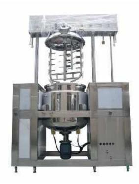
High speed shearing function is the main feature of automatic emulsifying mixer machine, which could mixing various of liquid product with continuous high speed mixing. Emulsifying mixing could help these different liquid material combine to one new condition that could not be mixed well normally. With continuous circulation mixing and emulsifying, you could get the high quality cosmetic cream product which already chemical component be rebuild.
