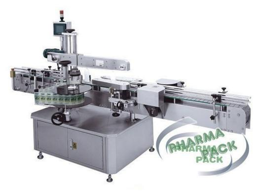
Label dispenser adopts servo motor to drive. Dispensing label implements closed- loop control. Label dispensing accuracy can be 0.2mm. Max. Label dispensing speed is 60 meters/min.
