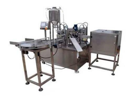
This filling and capping machine is used in cosmetics industry, and glue industry, such as nail polish, gel polish, glue, super glue. Our machine uses exclusive mechanical hand and the leading system to ensure the cap sit in the right position and realize a full automation.
