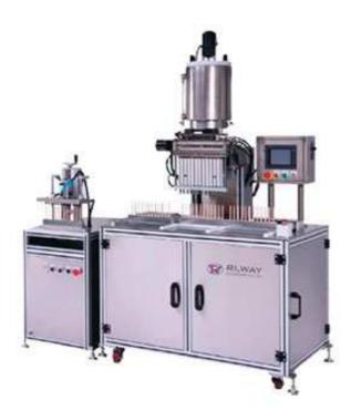
LS08-P3 is a pencil filling machine which specifically designed for filling high viscosity material. Such as eyeliners or eyebrow pencils.
