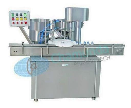
We bring forth precisely designed and developed Eye Drop Filling Capping Machine that is manufactured as per the industry standards. Highly demanded in pharmaceutical industries, these machines are famous for their capacity and consistent performance. The proposed series is tested for its quality before the final send off.
