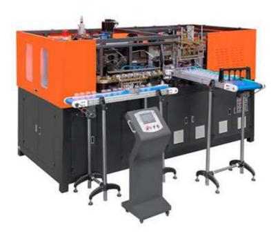
Plastic bottles cans blowing machine can blow bottles of different capacity, from 0.5 L to 3 L, used for the production of PET bottles of various shapes, such as mineral water bottle, cosmetic bottle, beverage bottles, cooking oils bottles, pesticide bottles, hot-filling bottles and other plastic containers. The Automatic PET bottle blowing machine shows the advantage of power saving, low defective rate, high speed, stability and easy operation.
