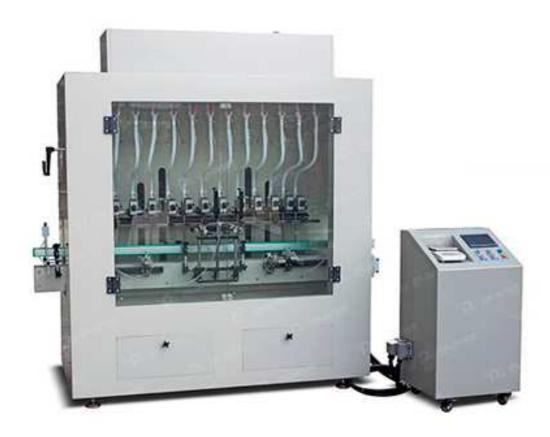
The disinfectant filling machine produced by Planet Machinery is a kind of filling equipment which is controlled by PLC and controlled by photoelectric sensor. This disinfectant filling equipment is mainly used for the filling of sanitizer liquid, disinfectant liquid, hand sanitizer, pharmaceutical alcohol.
