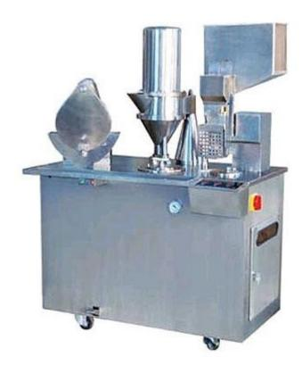
The machine is a new type of medicine packing machine with novel structure and attractive appearance. Under both electrical and pneumatic control and equipped with an automatic electronic counter and computer-controlled speed-adjusting device, the machine can accomplish the positioning, separation and locking etc. of capsules. In place of manual capsule-filling, it can reduce labor intensity and up to sanitary standards for pharmaceutics.
